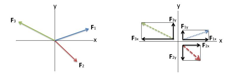
**Step 3**: Find the magnitude and angle of the resultant vector using the total of x and y elements.
