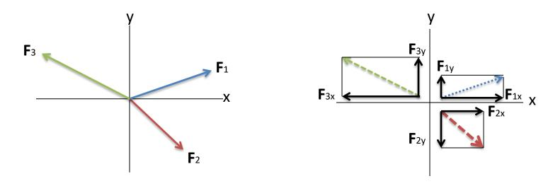
**Step 1**: Break up each force into its x and y elements.
