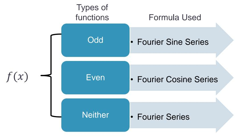
Note that: The odd and even function can also be solved using Fourier Series for interval [-L, L]
