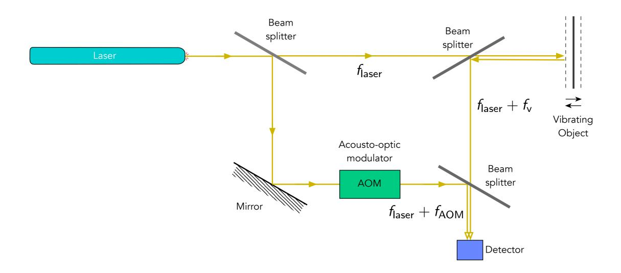
**Doppler effect: Principle of Laser Scanning Vibrometer**
