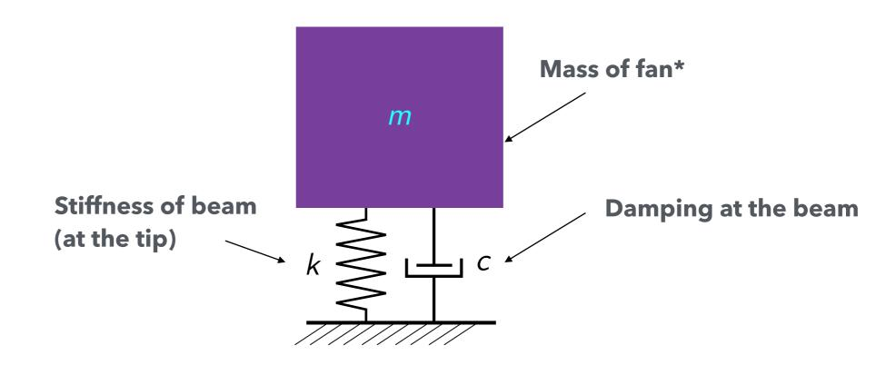
\*The beam is massless, otherwise the effective mass of the beam must be included in the mass component
