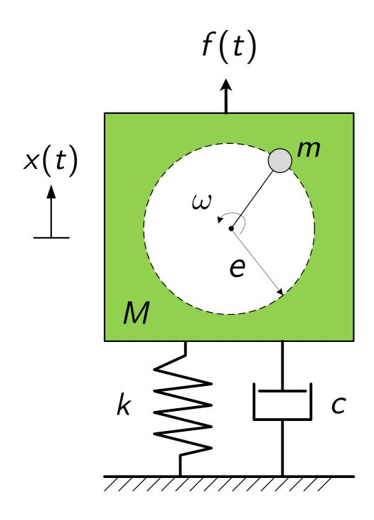
Centrifugal force produced by a rotating object:
