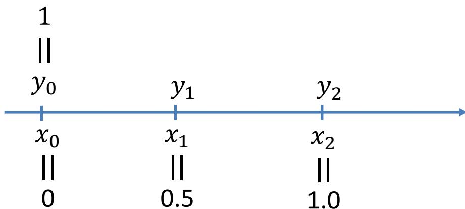
$$\begin{aligned} y_1 &= y_0 + \frac{1}{6} h(k_1 + 2k_2 + 2k_3 + k_4) \\ &= 1 + \frac{1}{6}(0.5)(1 + 2(1.5) + 2(1.625) + 2.3125) \\ &= 1.7969 \end{aligned}$$
