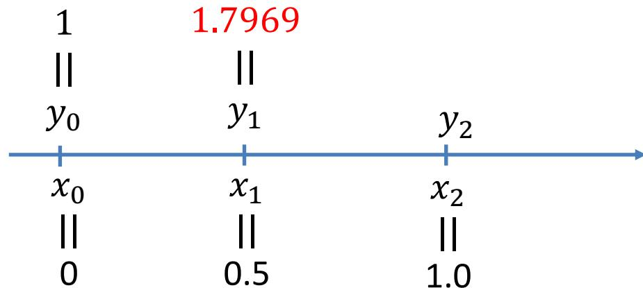
$$\begin{aligned} k_3 &= f\left(x_1 + \frac{h}{2}, y_1 + \frac{k_2 h}{2}\right) & k_4 &= f(x_1 + h, y_1 + k_3 h) \\ &= f(0.75, 2.5772) & &= f(1, 3.4605) \\ &= 3.3272 & &= 4.4605 \end{aligned}$$
