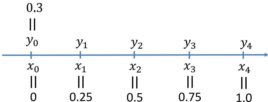
$$\begin{aligned} y_1 &= y_0 + \frac{1}{6} h(k_1 + 2k_2 + 2k_3 + k_4) \\ &= 0.3 + \frac{1}{6} (0.25)(0.3624 + 2(-0.1865) + 2(0.0725) + (-0.4560)) \\ &= 0.2866 \end{aligned}$$
