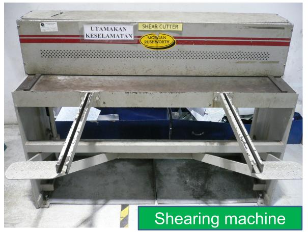
A shearing machine is used to cut along a straight line of sheet metal.
