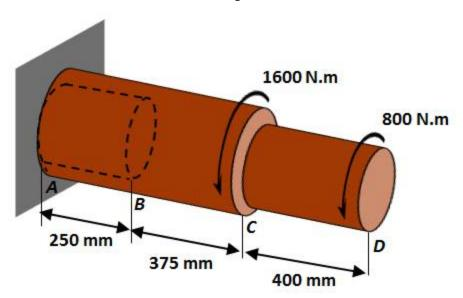
Rod *ABC* is made of brass (G= 39 GPa) with outer diameter of 60 mm. The portion rod *AB* is hollow has an dinner diameter of 40 mm. The rod *ABC* is bonded to aluminum rod *CD* (G= 27 GPa) with diameter of 36 mm. Determine the angle of twist at end *D*.
