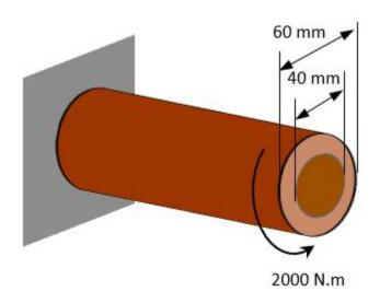
For the hollow and loading shaft shown, determine:
