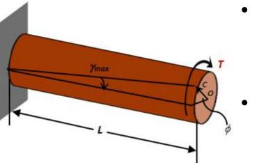
The relationship between angle of twist and maximum shearing stress:
