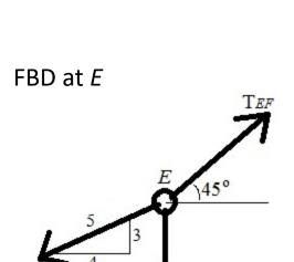
Assume that all cables are in tension. Given  $W_A = 20 \text{ N}$
