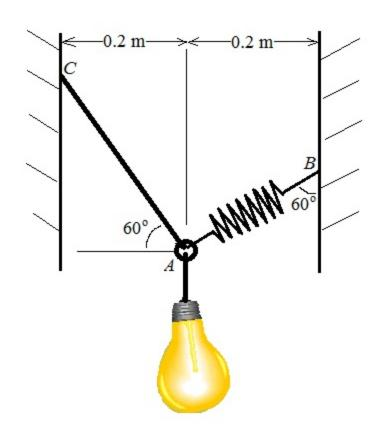
Given a lamp as shown in figure with mass 0.4 kg which is suspended by cable AC and spring AB.
