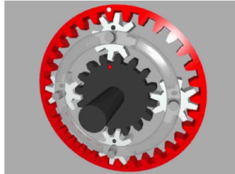
PLANETARY OR EPICYCLIC GEARS
